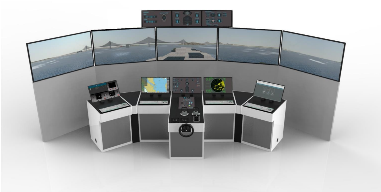
Figure 1 – Ship Bridge Simulator – proposed configuration
