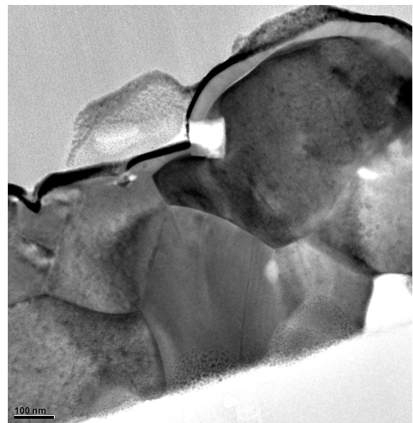
Figure 2: The microphotograph of the cross-section of the chemically deposited PbSe-based photoresistor obtained with the help of the high-resolution transmission electron microscopy
