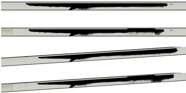
Figure 3: Smoke Movement for Four 5 MW Fire Scenarios after 100 s to the Fire
