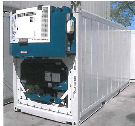
Figure 2: Refrigerated container with integrated refrigeration and power supply generator 2
