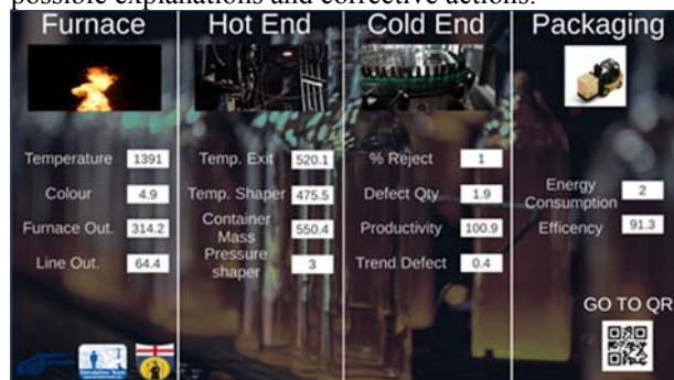
Figure 3: Mobile application displaying main plant indicators
