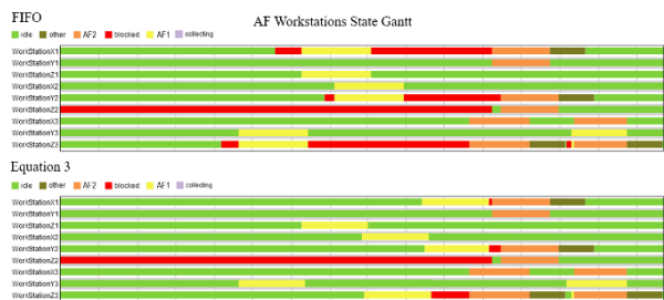
Figure 8. Gantt charts of AF with FIFO (above) and (3) (below) dispatching rules in scenario 3.
