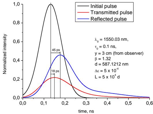
**Figure 6.** Time dependence of the averaged intensity in the reflected (blue) and transmitted (red) signals for the interference filter exposed to ultrashort Gaussian light pulse (black).
