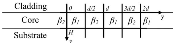
**Figure 1.** The structure of the planar waveguide with the phase grating written.
