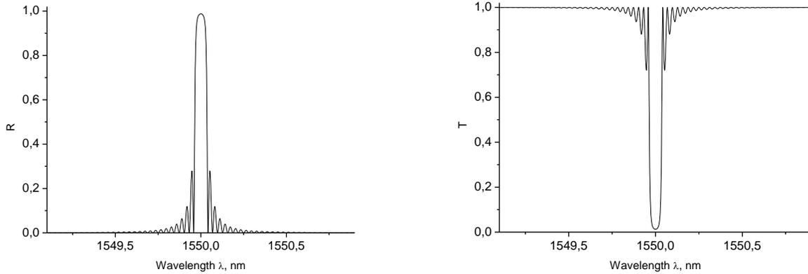
**Figure 4.** Reflectivity  $R$  and transmittivity  $T$  coefficients of the grating with period  $d$  and length  $L$  as a function of incident wavelength  $\lambda$ .  $d = 0.58712 \text{ MKM}$ ,  $L = 5 \times 10^4 \times d$ ,  $\Delta\varepsilon = 1 \times 10^{-4}$ .
