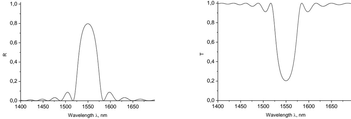
**Figure 5.** Reflectivity  $R$  and transmittivity  $T$  coefficients of the short grating with period  $d$  and length  $L$  as a function of incident wavelength  $\lambda$ .  $d = 0.58712 \text{ MKM}$ ,  $L = 50 \times d$ ,  $\Delta\varepsilon = 0.05$ .
