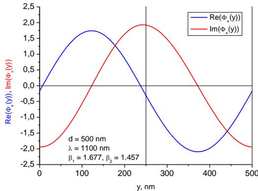
**Figure 3.** The graph of Bloch function outside the resonance (for  $\lambda = 1100$  nm). The parameters of the model are shown in the insertion.
