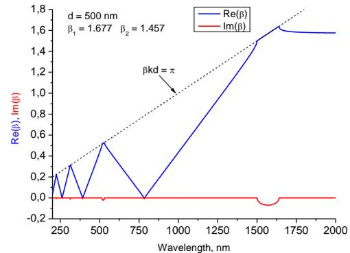
**Figure 2.** The  $\tilde{\beta}$  dependence of the wavelength  $\lambda$  for one of the solutions of dispersion relation (5). The other solution is obtained by changing the sign of  $\tilde{\beta}$ . The parameters of the model are shown in the insertion.
