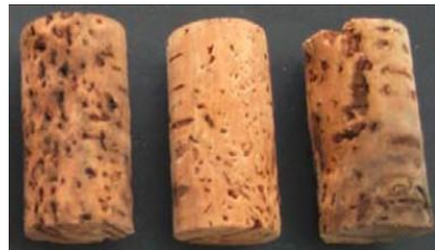
Figure 4. 24x44 mm cork stoppers subjected to a treatment of 127 °C - 1.5 bar for 45 min.
