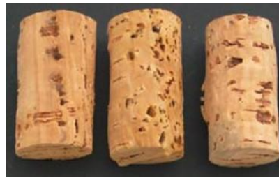
Figure 3. 24x44 mm cork stoppers subjected to a treatment of 120 °C - 1 bar for 45 min.
