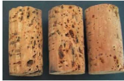
Figure 2. 24x44 mm cork stoppers subjected to a treatment of 110 °C - 0.5 bar for 45 min.
