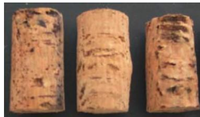
Figure 5. 24x44 mm cork stoppers subjected to a treatment of 133 °C - 2 bar for 45 min.
