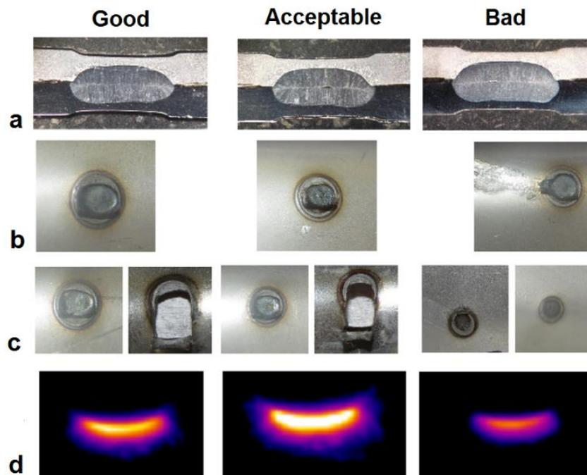
Figure 4. Defined classes to label the images of the dissimilar joints a) presence of pores, b) presence of expulsion, c) failure mode. d) IR image.
