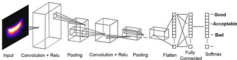
Figure 1. Basic structure of a CNN.
