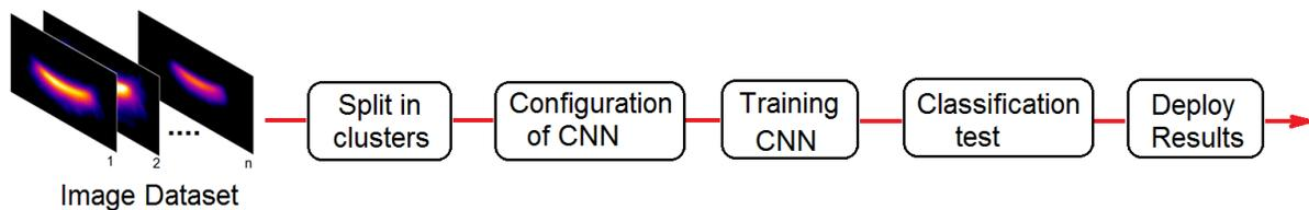
Figure 2. Diagram of CNN network approach implementation.
