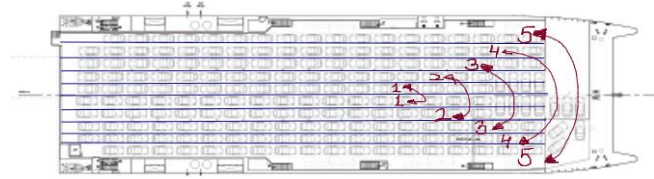
Figure 3. Diagram of lanes in a RoRo vessel
