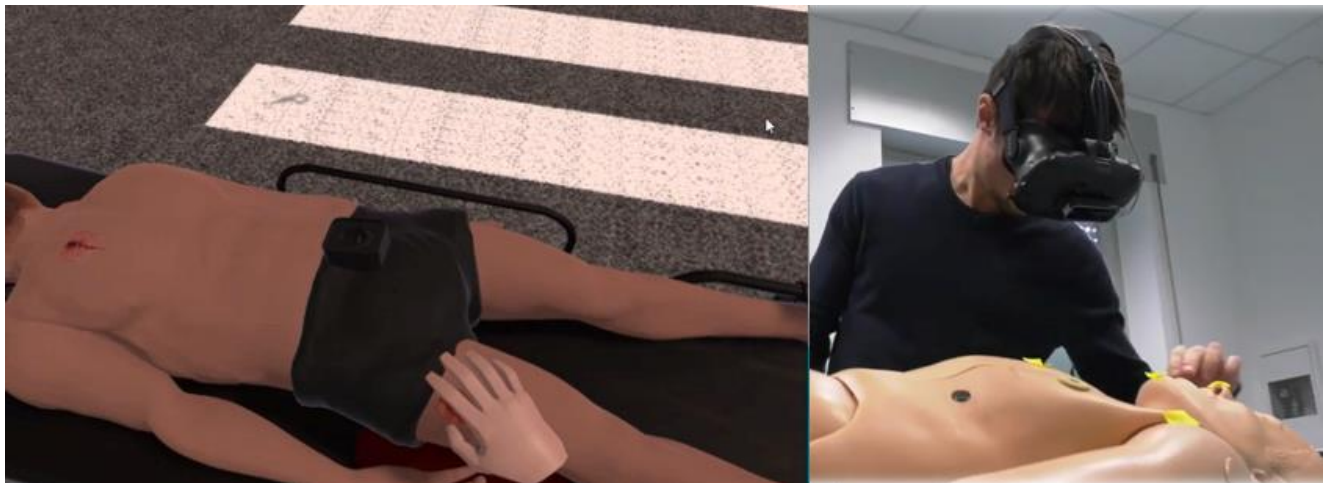
Figure 4. MR application for first aid training. Left: virtual reality representation of the manikin located in an urban environment. Right: real world, the user, through the head mounted display, sees the medical emergency on the left. With the real manikin he can physically interact with the simulated patients, while seeing a virtual representation of his own hands.
