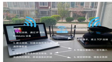
Figure 9. Schematic diagram of information transmission between PC and Hololens 2
