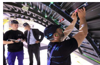
Figure 7. MIRA/SART for structural bracket detection
