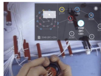
Figure 4. Boeing's electronic circuit arrangement based on AR glasses
