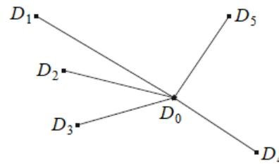
Figure 1. The localization of the signal source by a set of 5 sensors
