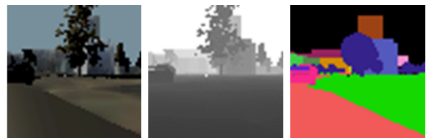
Figure 1. Visual observation examples taken from the simulator (from left to right): raw agent camera, depth agent camera, and segmentation agent camera.
