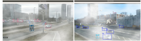
Figure 6. Object detection with fog filter=50% and 70%
