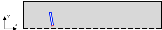
Figure 3. Schematic representation of the computational domain. Width is 1.64 m and height is 32 cm. The bottom horizontal dashed line represents a conveyor. The air blade (delimited by blue and red lines) is 16 cm long and is oriented 10^\circ relatively to the vertical axis, 1 cm above the conveyor. The end of the air blade (red line) sizes 100 \mu\text{m} .
