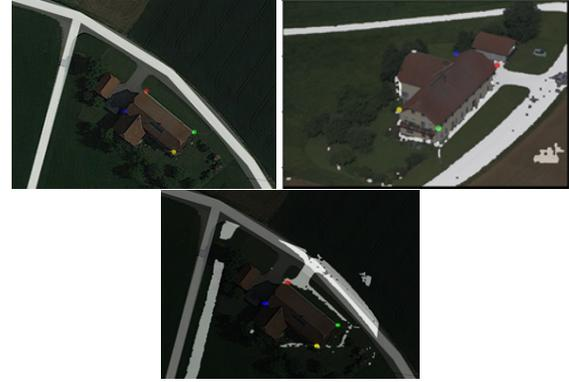
**Figure 12.** Registration based on 4 manual landmarks precisely defined on the building roof.
