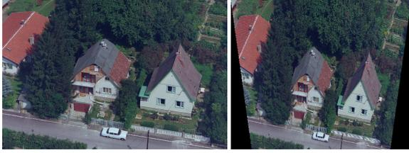
Figure 6. Test runs on image 10 of sequence "A 7 058 11" from 2012. The original aerial image and the result after rectification.
