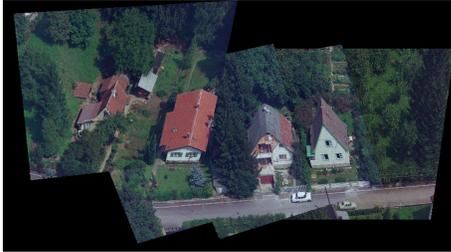
Figure 7. Test runs on images of sequence "A 7 058 11" from 2012. With rectified images 6, 10, 11 and 12 image stitching of the particular street of houses becomes possible.
