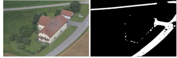
Figure 8. U-net based segmentation allows solid identification of the streets as target structures. Despite occlusions, the particular street fragments are provided at high quality with only few FP scatter present.
