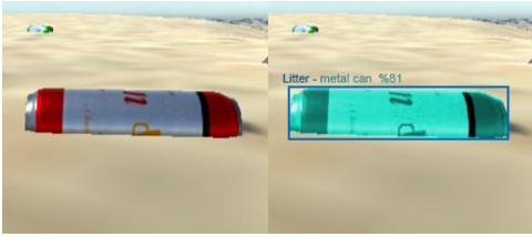
Figure 6 The picture of a metal can 3D-object belonging to the Virtual Framework (left) properly classified by the DeepLabv3+ image segmentation software (right), that has successfully recognized the litter class with an accuracy of 81%
