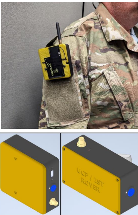
Figure 1. View of a physically worn Rover Module (top) and CAD renderings of Rover Module variations (bottom).
