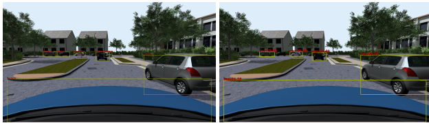
Figure 7. Two examples of the inference run with YOLOv3 Redmon and Farhadi (2018), both show instances where the cars are being miss detected in the lower resolution dataset. Images on the left have the original resolution of 2560x1440 and images on the right of 1440x720. Virtual scenario and sensor data generated using VEROSIM VEROSIM and the framework presented in Thieling and Rosmann.
