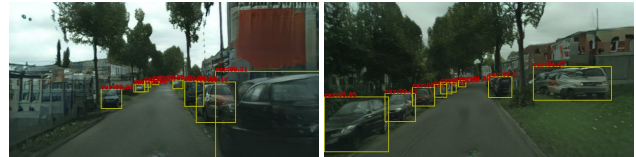
Figure 8. (top) Precision vs Recall curve for car detection from YOLOv3 Redmon and Farhadi (2018) on the vidzvid Wang et al. (2018a) output using semantic images from VKITTI2 Cabon et al. (2020); Gaidon et al. (2016), giving an average precision of 20%. (bottom) Two examples of the results.
