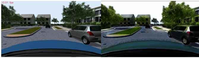
Figure 3. Example of the development in Thieling et al. (2019) applied to our simulation pipeline. Color transfusion from vegetation is present in some objects due to the distribution of trees and houses in the limited real dataset used in that research. Virtual scenario and sensor data generated using VEROSIM VEROSIM and the framework presented in Thieling and Rosmann.
