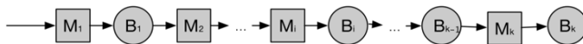
Figure 1. Serial flow in a production line composed of K machines (boxes) and K buffers of capacity B_i .
