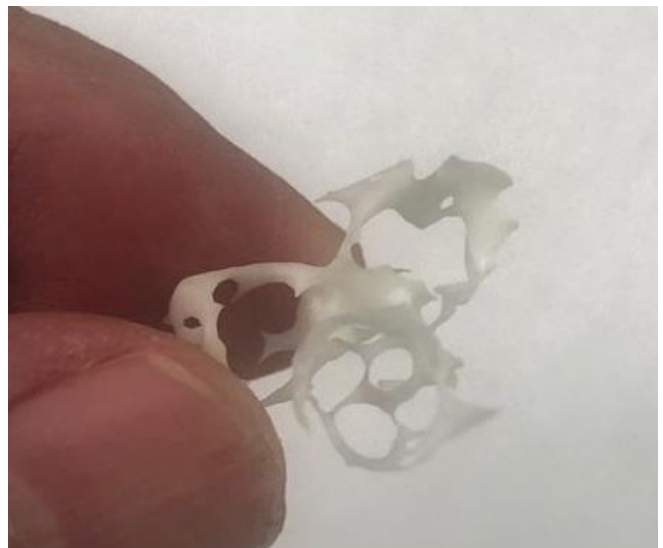
Figure 15. Close-up of the three 3D printed resin Zephyr valves.
