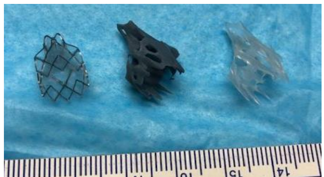
Figure 16. Comparison of resin valve with actual Zephyr valve.
