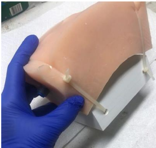
Figure 8. Cast part connected to 3D printed support structure.
