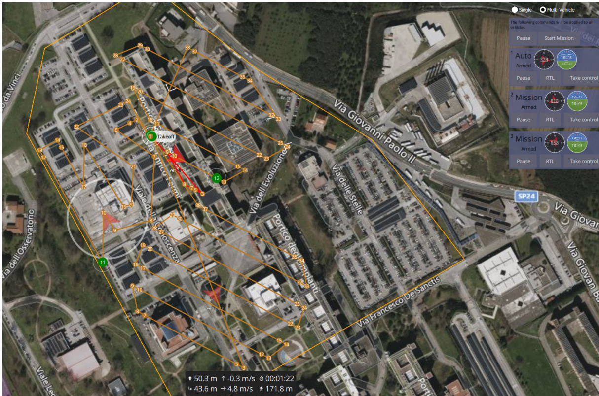
Figure 3. QGroundControl view of a simulated mission with three drones flying over the University of Salerno.
