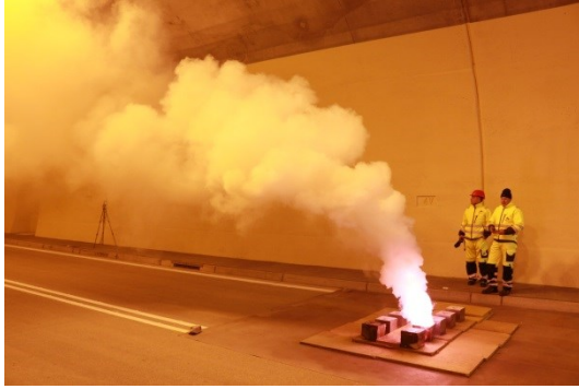
Figure 3. Smoke tests in the Polana tunnel.
