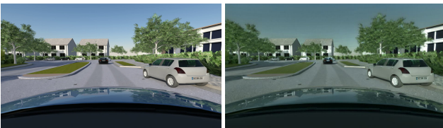
Figure 10. Cross-inferences obtained with the model trained with GTA V dataset: starting simulated image (left) compared to the corresponding resulting inference obtained with the model trained for 1M iterations (right).
