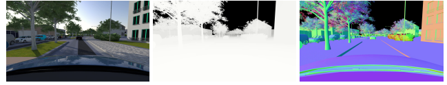
Figure 2. Ray-tracing simulated color image (left), corresponding ground truth depth map (middle) and ground truth surface normals map (right), all generated with the VTB in VEROSIM.
