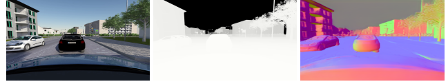
Figure 3. Ray-tracing simulated color image (left), and corresponding ground truth depth map (middle), both generated with the VTB in VEROSIM, and surface normals map generated with the AI model (Eftekhari et al., 2021).
