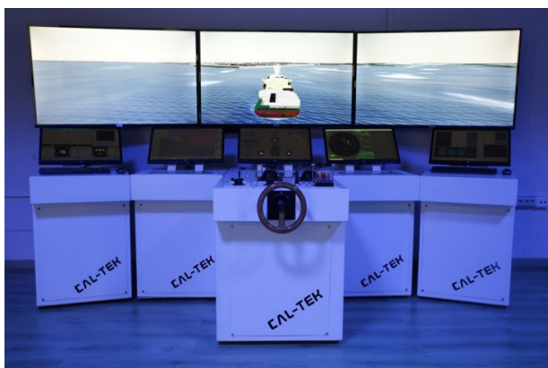
Figure 2. Ship Bridge Simulator
