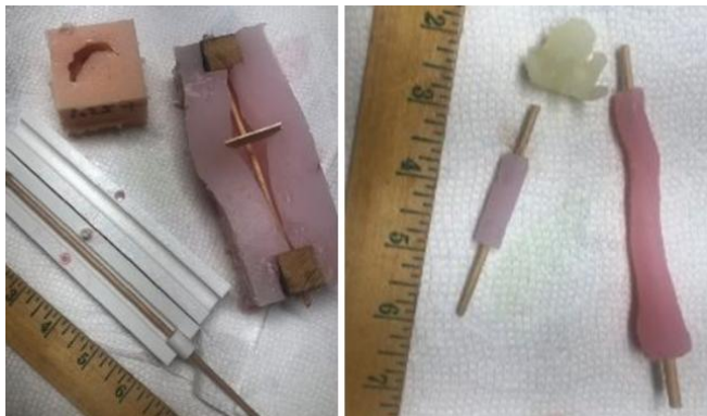
Figure 7. Molds (left) and cast parts (right) of ovary, fallopian tube and ligament.
