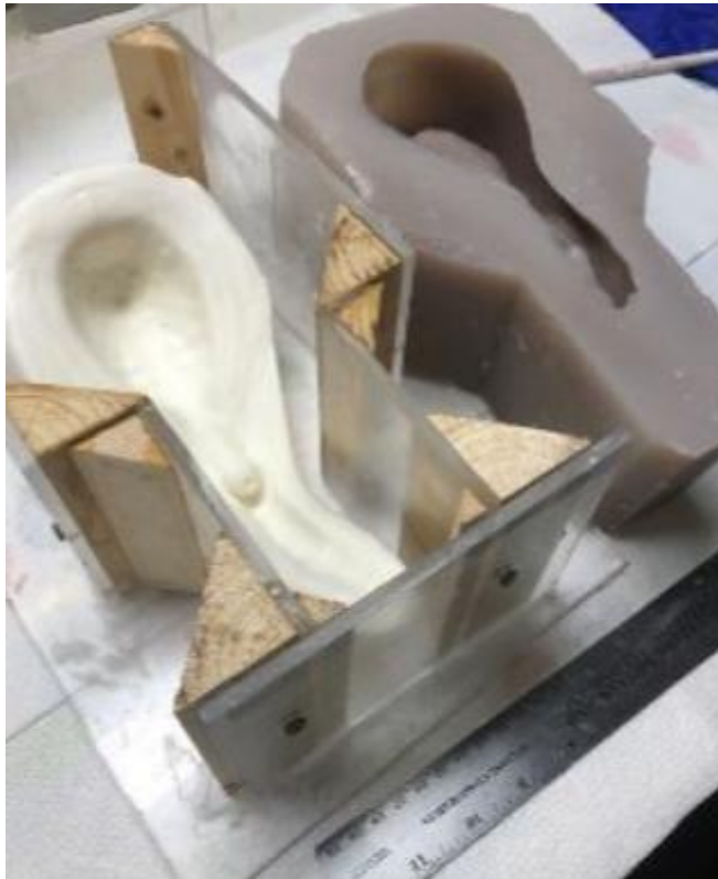
Figure 6. Uterus pattern in mold box (left) and finished silicone rubber mold (right).
