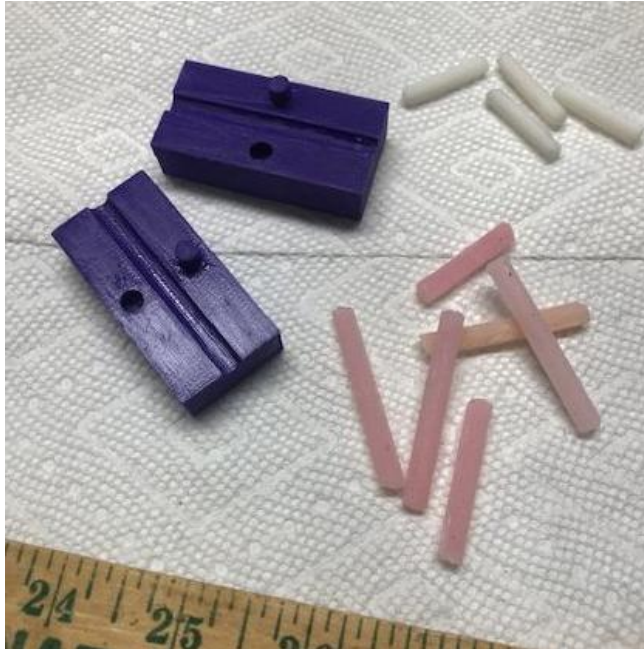
Figure 4. Clitoris two part mold box (left) and silicone rubber castings (right).
