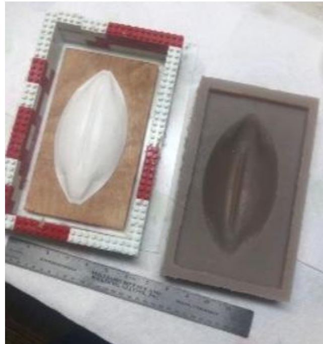
Figure 2. Labia majora PLA pattern in mold box (left) and completed silicone rubber mold (right).
