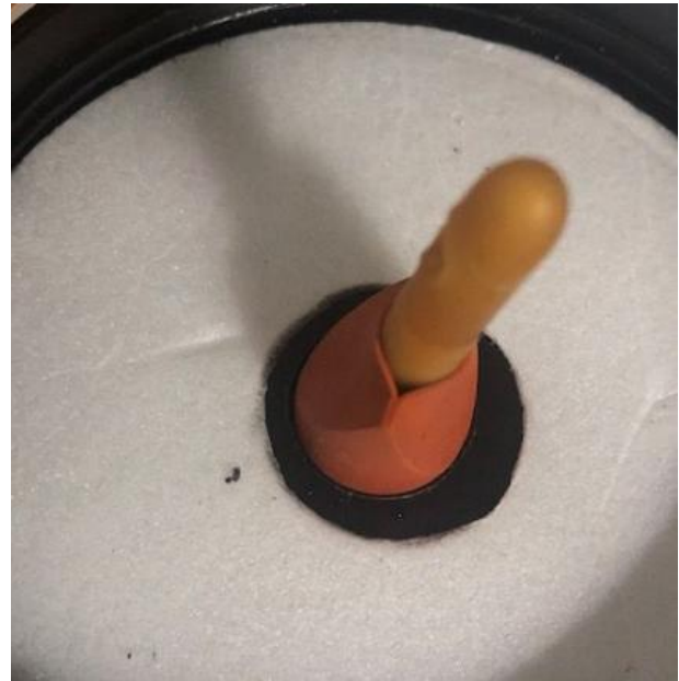
Figure 5. Catheter passing through the duck bill valve.
