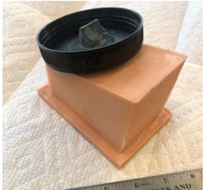
Figure 3. Cast block of Dragon Skin with the urethra and vagina. Duck bill and bottle cap glued to Dragon Skin block
