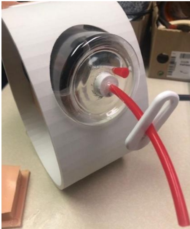
Figure 7. Addition of tubing to refill the bladder bottle.
