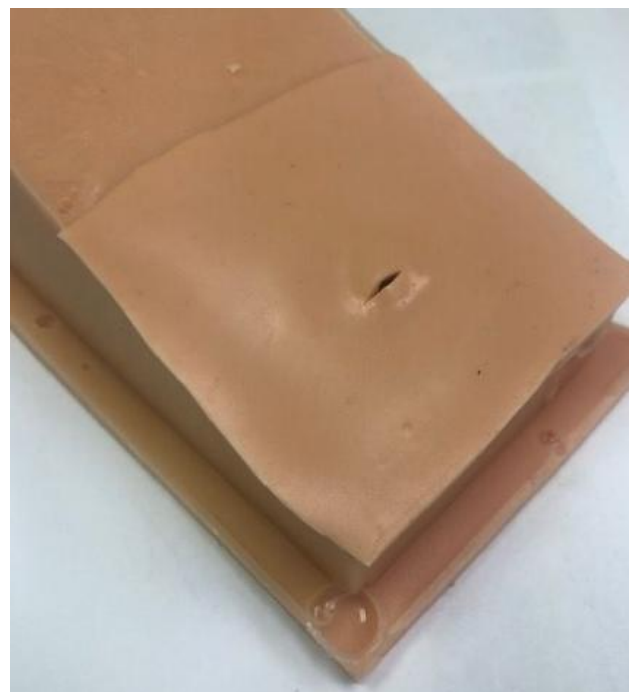
Figure 6. 1.5mm thick membrane installed over the block of Dragon Skin.
