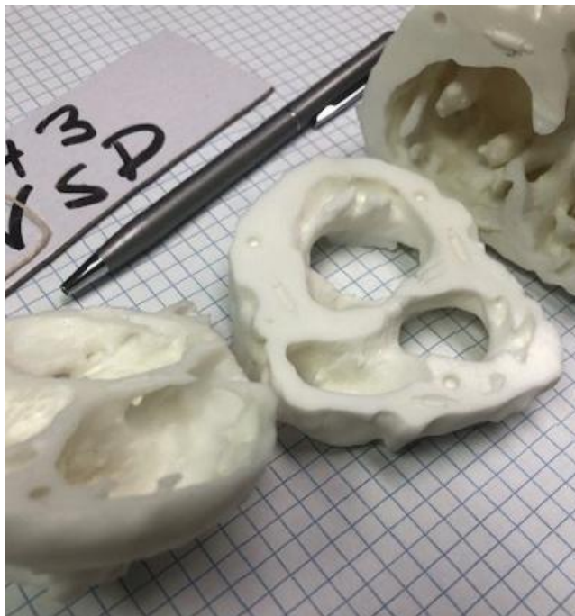
Figure 8. Axial slices of Heart3 with VSD (left slice) using resin.
