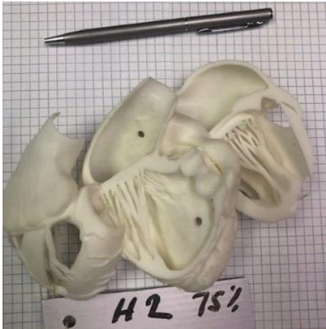
Figure 7. Slices of Heart2 with added ASD and VSD using PLA filament.
